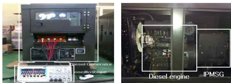
Fig. 7. Experimental set-up for the diesel generator
