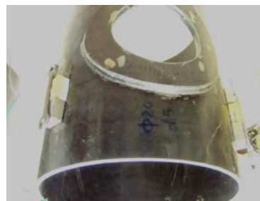
Figure 2: Specimen simulating a T-joint with reinforcing plate.
