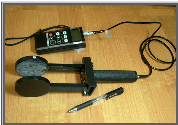
Fig.7. Device for eddy-current control BD-1
