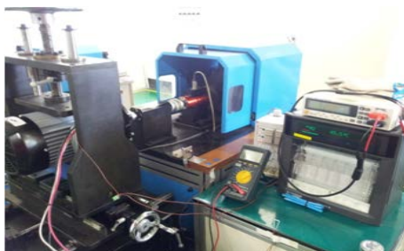
Figure 5 (a) Dynamo setup to test the LSPM
