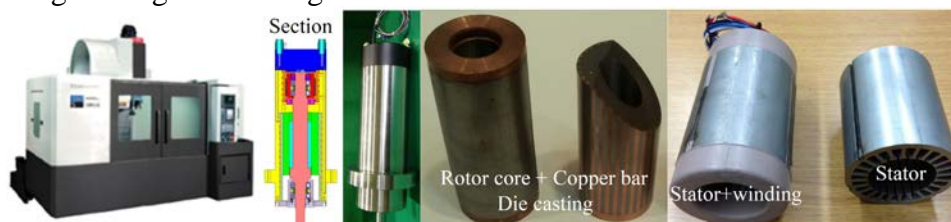
Figure 1: The configuration of prototype, high speed and high efficiency induction motor
