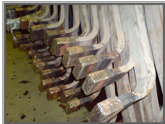
Fig.2. Stator bars with brazed clamps
