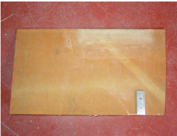
Figure 2 Left : composite part with hole type IQI,
