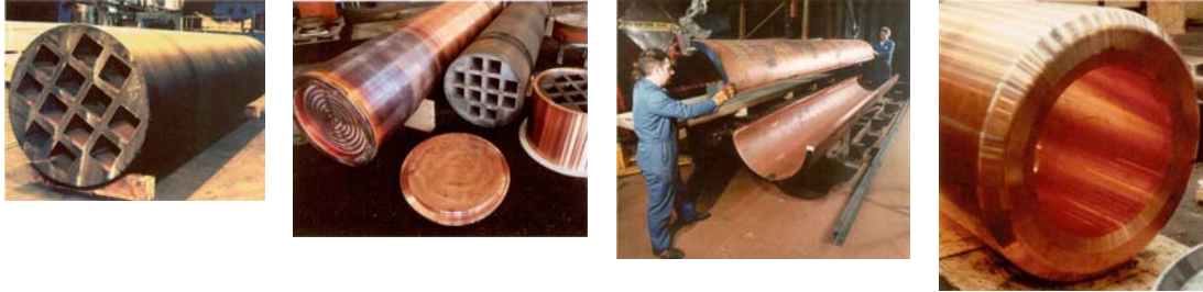
Fig. 3: Construction of the copper canister
